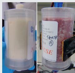
Fig. 1: Miniaturized CytoSorb columns (scale 1:5; V_{ads} = 60 mL) with polyvinylpyrrolidone-coated polystyrene-divinylbenzene copolymer adsorbent prior to (left) and during recirculation of human whole blood (right)
