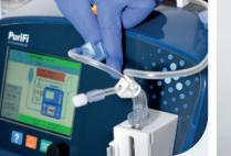
Insert hydrophobic filter to metal connector.
