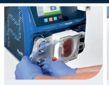
Confirm pump segment and inline transducer placing
