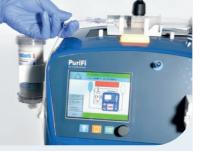
Connect heparin syringe to heparin line and place syringe in slider.
