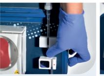
Insert **blood return line** in air sensor and automatic clamp.
